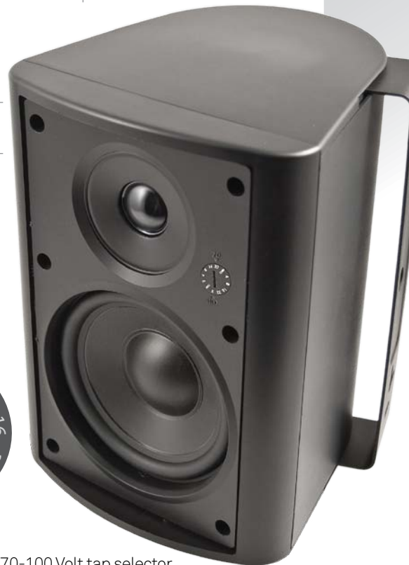
Front mounted 70-100 Volt tap selector switch with bypass setting for 8-ohm applications Tap Selection Settings: 2, 4, 8, 16, 32W (70V) & 4, 8, 16, 32W (100V)
