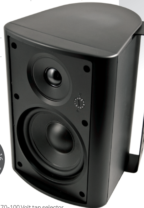
Front mounted 70-100 Volt tap selector switch with bypass setting for 8-ohm applications Tap Selection Settings: 2, 4, 8, 16, 32W (70V) & 4, 8, 16, 32W (100V)
