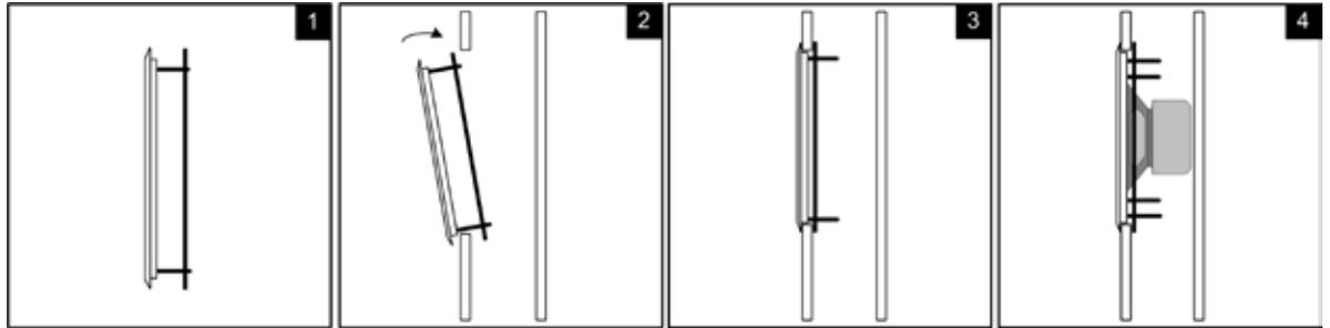
or loose insulation, it is important to prevent the insulation from entering the back of the speaker. This can be accomplished by placing a batt of fiberglass insulation over the back of the speaker.
