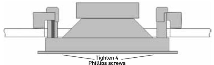
If the speaker frames are to be painted, either before or after installation, use the paint-mask (the inner cardboard disc) to cover the speaker driver(s) to prevent damage. DO NOT PAINT THE GRILLE AND FRAME ASSEMBLY TOGETHER. The grille should be painted separately. Use thin coats and thin the paint as necessary to avoid clogging the perforations with excessive paint.
