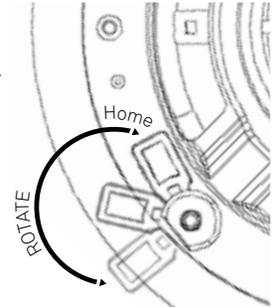
Verify that the speaker fits properly into the cut-out. If the hole should have been cut a little too large the flange on the speaker should cover this. Remove the speaker from the hole.
