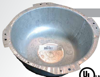
PE-8 Steel Plenum Dome for Fire Rated applications. Includes EMT knock-outs for easy twist lock assembly when using with PB-6 & PB-8. Use with T-bar bridge in drop ceilings.
