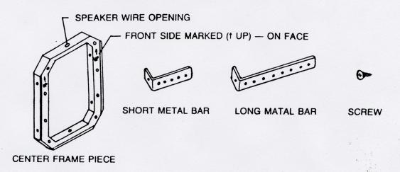
STEP 2. STABLE THE METAL BARS WITH THE CENTER FRAME PIECE USING THE LONG SCREWS.
