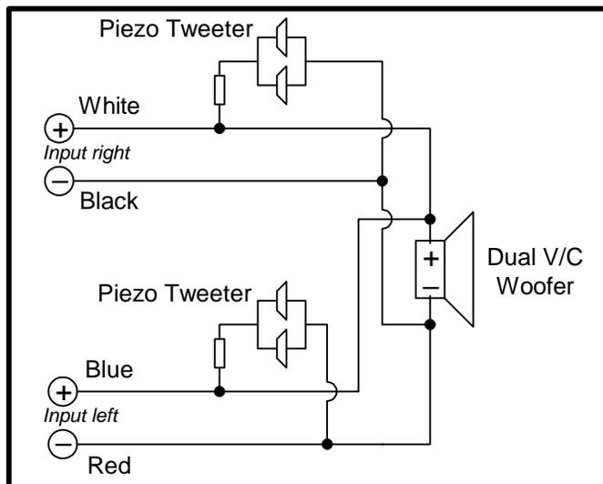
If your unit does not have four tweeters mounted to the metal ring and it does have four connection wires, then you have the newer model and the tweeters are behind the black foam where you can't see them. All updated models use this wiring scheme:
